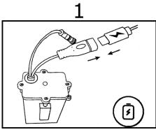
Please ensure batteries in Host are fully charged after receiving the goods. Charge time is around 4-5 hours, the light will be on solid blue when fully charged.
