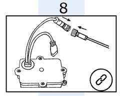
Connect the flush button to the Host, ensure you screw collar tight once plugged in. You can now carefully place the lid back on your cistern.
