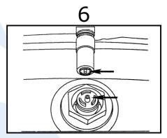
Install flush button into hole on toilet lid, then connect the extension base, ready for placement back onto the toilet cistern.
