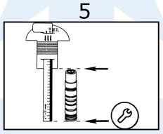
Use the blocks to assemble an extension base as long as the measured ruler from Step 4.
