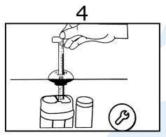
Take out the ruler included in your package, and measure the distance between the toilet tank fluid and the flush valve.
