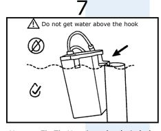
Hang or Zip Tie Host into the drain hole of the toilet cistern, do not to get wet above the hook. Please also ensure rubber stopper is installed on Host, to prevent water getting inside.
